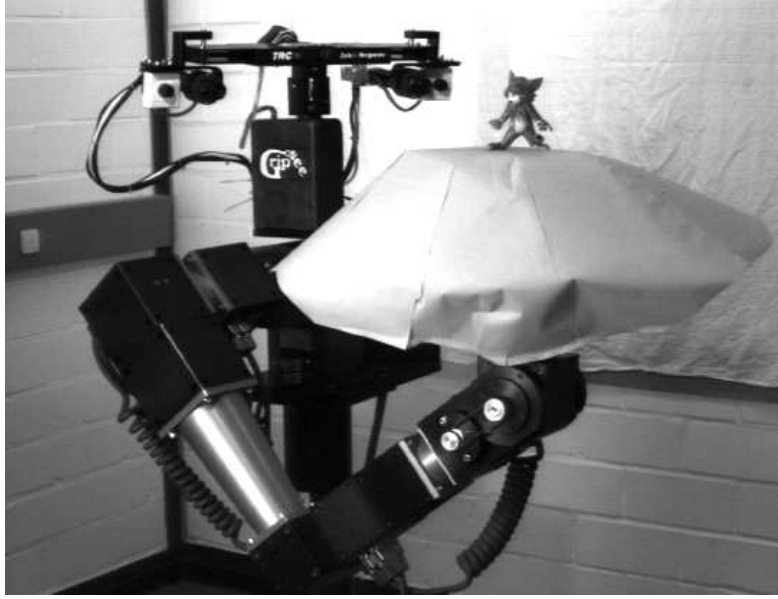
Figure 3.3: Robot Scene. The robot arm has the squared timber on which the “Tom” object is fixed in its gripper. The timber and the gripper are covered by a gray background. (For the recording of the images not the displayed stereo cameras were used but another single camera.)
