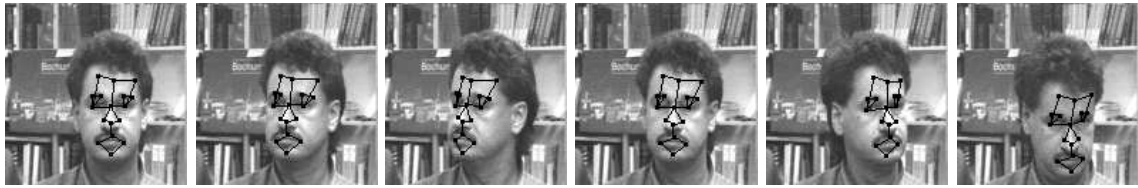
Figure 3.9: Tracking Local Object Features. These results taken from Maurer and von der Malsburg [36] show the views 1, 10, 20, 30, 40, and 50 of a tracked sequence.
