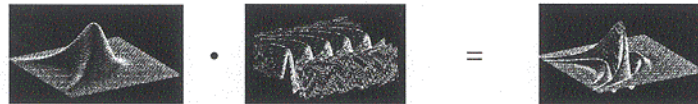
Figure 3: A banana wavelet is the product of a curved Gaussian G^{\vec{b}}(x, y) and a curved wave function F^{\vec{b}}(x, y) (only the real part of the kernel is shown).
