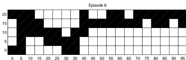
Figure 10 Key views of the learned scan path after episode 8. This path yields the smallest total error of 0.030.
