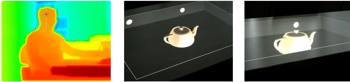
Results from a Projector-Camera Project. Left: Colored depth image with detected 3D head position of a user. Middle and right: Two different views of a projected object depending on the user's head position. Images from Garstka & Peters, "View-dependent 3D Projection using Depth-Image-based Head Tracking", PROCAMS 2011.
